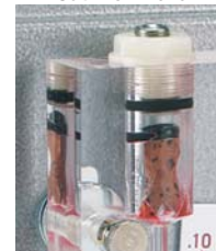
Fig. 7-5. Type "c" with shipping plugs in place.
